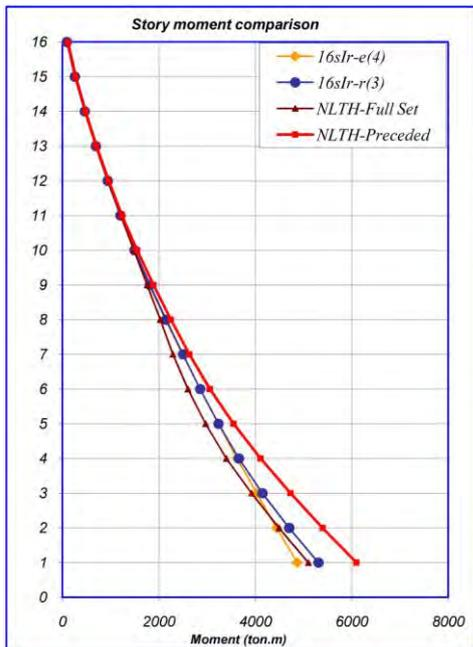
Fig. 7 Comparison of story moment between NLRHA and MPA using eigenvectors and LDR vectors
