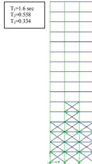
Figure 1 Irregular 16-story frame model that has been used in the application of MPA with LDR
