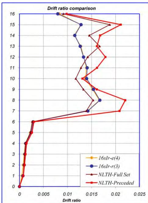
Fig. 8 Comparison of drift ratio between NLRHA and MPA using eigen-vectors and LDR vectors
