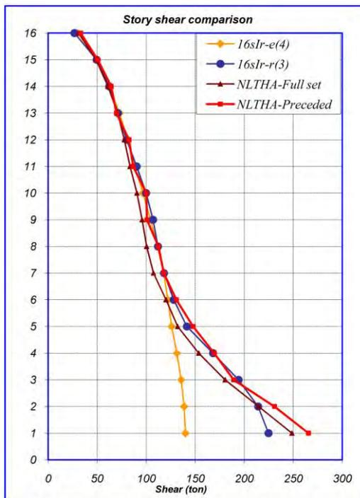
Fig. 6 Comparison of story shear between NLTHA for full and selected record set and MPA using eigenvectors and LDR vectors
