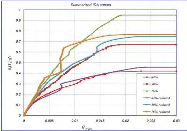
Fig. 3 Comparison of full and reduced data set summarized IDA curves: first spectral acceleration vs. maximum inter-story drift.
